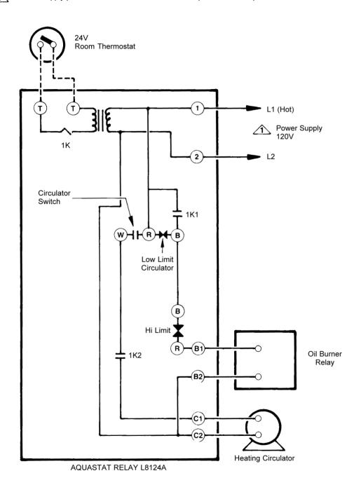
WIRING ARRANGEMENT FOR "NP" BOILER CONTROLLING OPERATION OF BOILER AND CIRCULATOR
