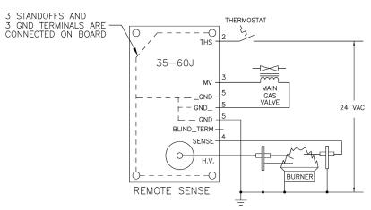
BLIND\_TERM: NO CONNECTION TO CONTROL PLACE HOLDER FOR ANY LOOSE LEAD.
